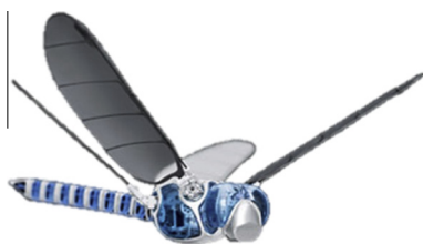
Fig. 18. Festo BionicOpter – inspiration dragonfly flight [286].
