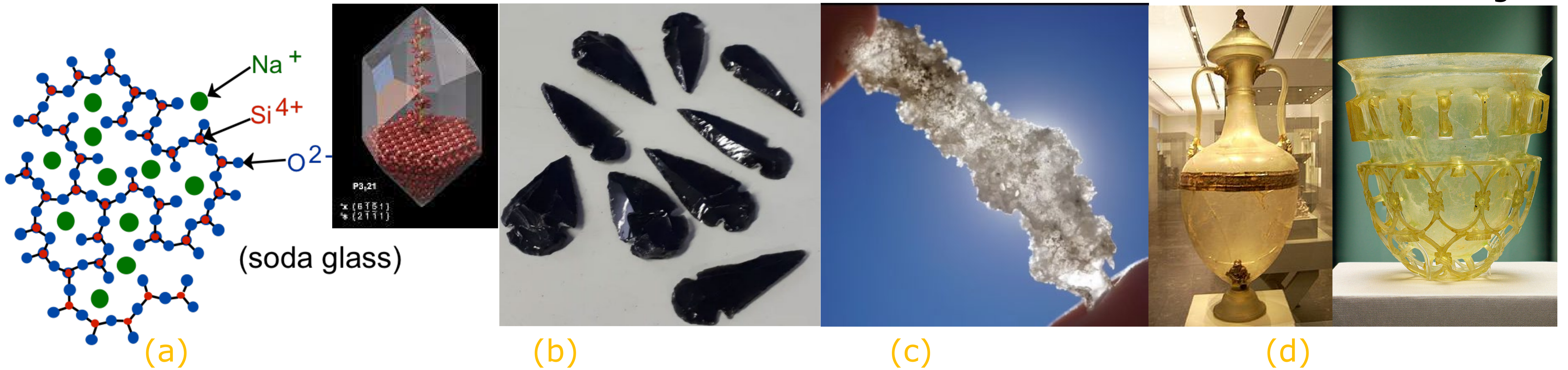
Figure 1: (a) typical glass amorphous solid liquid structure compared to quartz crystal; (b) Obsidian glass used for arrow heads; (c) A fulgurite (“frozen lightning”) Quartz glass found on a beach; (d) Ancient Greek Glass Amphora circa 150 BC (left) and 4 th Century Roman Glass Cage Cup AD(right)
