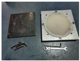
**Step 12** – Carefully remove the silicone insert using a big flat head screwdriver. Slip it down in between the frisbee and the silicone and lever it out. It might be easier with 2 screwdrivers.
