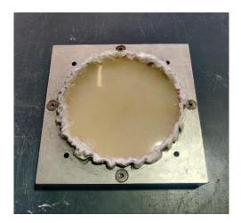
**Step 9** – Bolt the steel plate on to the top off the silicone using the M8 bolts and matching nuts to create pressure in the tool. You want to make sure that the steel plate is aligned using the alignment marks as shown below. Make sure that you tighten the bolts evenly, a good way to do this is to count the exposed threads . **Don't** over tighten the bolts because you will damage the silcone, it should be tight but don't force it.
