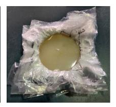
**Step 8** - Once you have the silicone in the tool make sure that you can see the patterned fabric poking out of the tool **on all sides** as shown below. This will ensure that you have aligned the fabric correctly. Then trim off the excess fabric with scissors or a knife, you want to get as much off as you can to expose the 4 holes in the tool, it should look like the picture below (Right).
