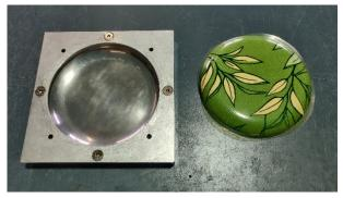
**Step 15** – Trim the excess plastic off around the tool part line using a sharp knife.
