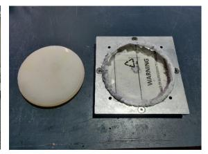
**Step 13** – Trim the exposed part of the frisbee with a sharp knife, use the tool surface as a guide as to not cut the actual part.
