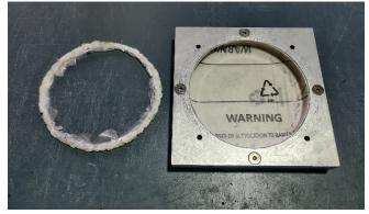
**Step 14** - Then unscrew the countersunk bolts and separate the tool to retrieve the part.
