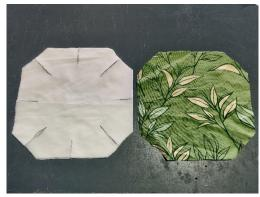
**Step 3** – Lay 1-2 sheets of clear LDPE (depending on thickness), that is bigger than the template, as the first layer of the layup. This will be the top surface of the frisbee so make sure that is it clean and free of any contamination. Then lay your patterned fabric, **pattern DOWN**, on top of the plastic as shown below.
