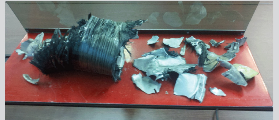
Filament Wound Tank After Burst Test
