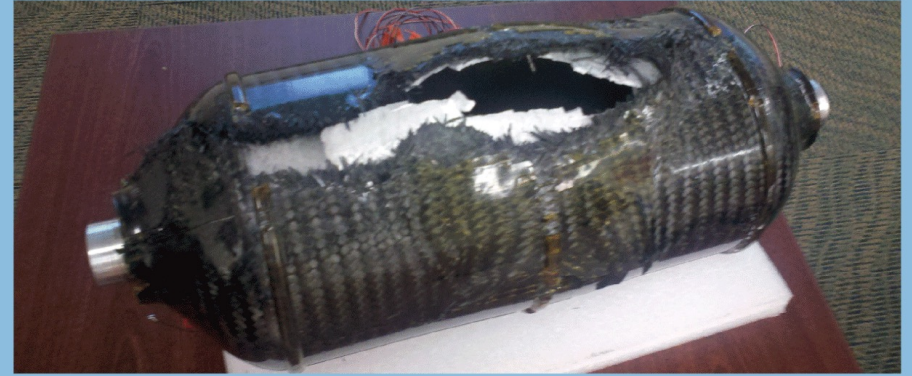
Braided Tank After Burst Test
