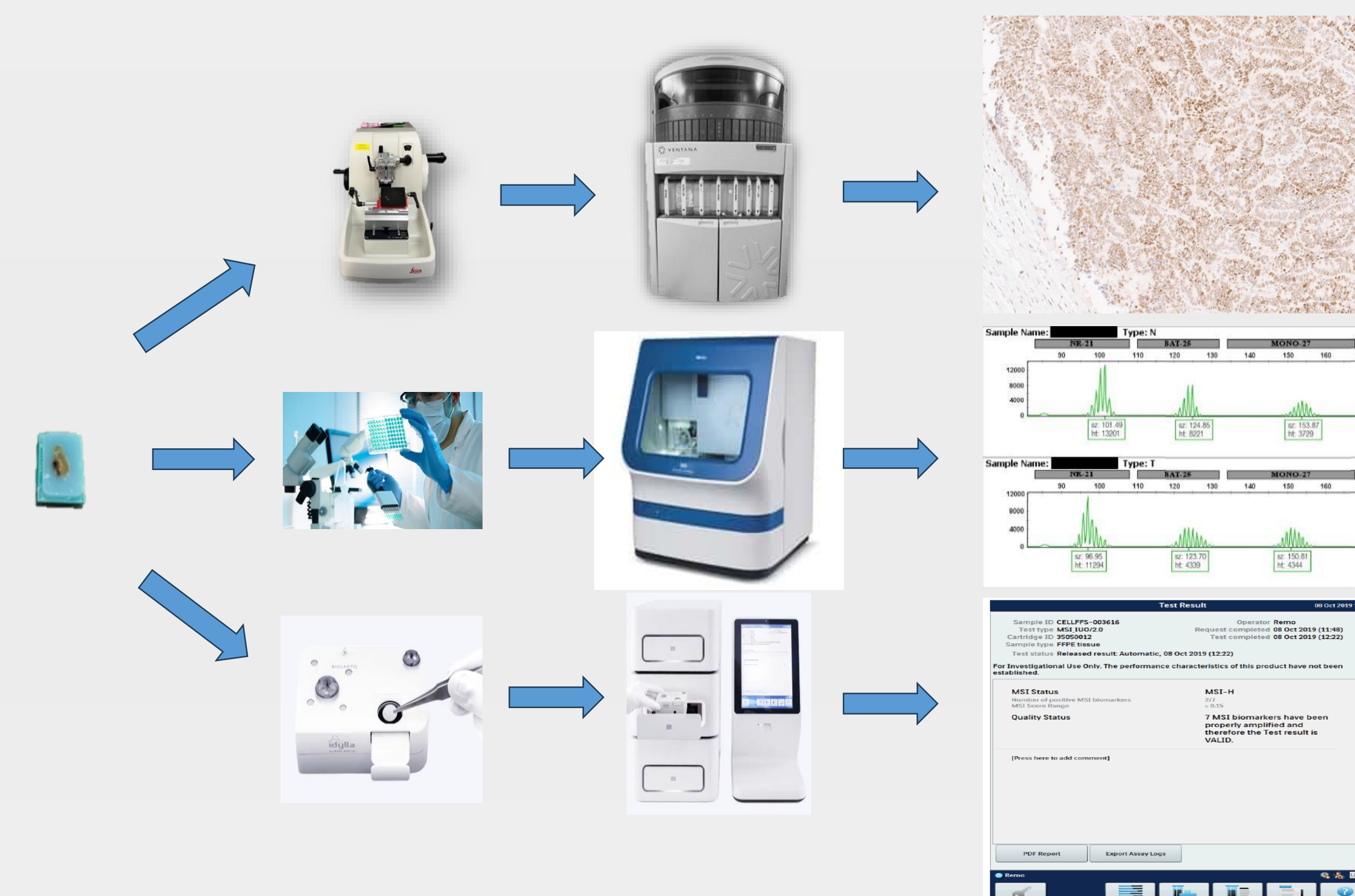
Figure 2: Currently available FDA-approved testing workflows for the identification of dMMR/MSI in screening for Lynch Syndrome: VENTANA or BOND MMR panels (top), OncoMate™ MSI Dx (center), and Idylla™ MSI Test (bottom)
