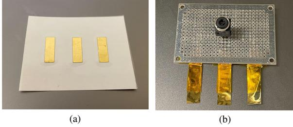
Fig. 1: E-Tattoo (a) Electrodes and (b) Reusable Connector
