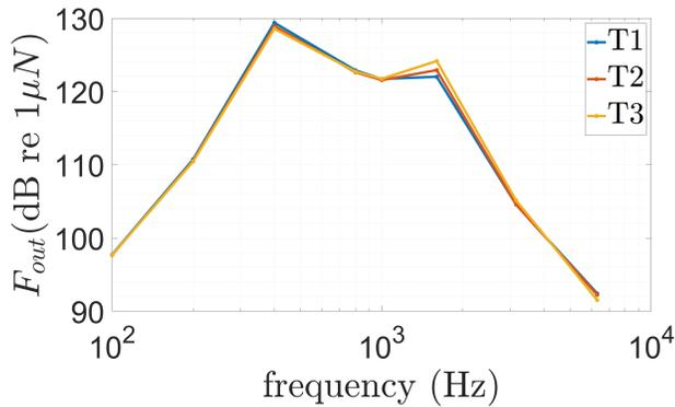
Fig. 2: Calibration of the three used transducers T1, T2 and T3 for  $f \in [100, 200, 400, 750, 1500, 3000, 6000]$  Hz and  $a = 0.5$  V
