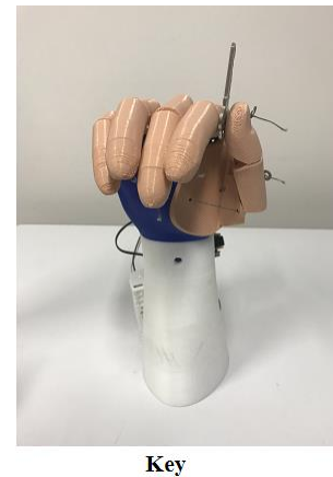
Fig. 9. Lateral grasp of a key. Please note that the thumb is in the non-opposed position for this grasp.
