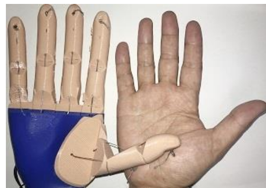
Fig. 6. The 3D-printed UoW/ACES prosthetic hand and a real human hand.
