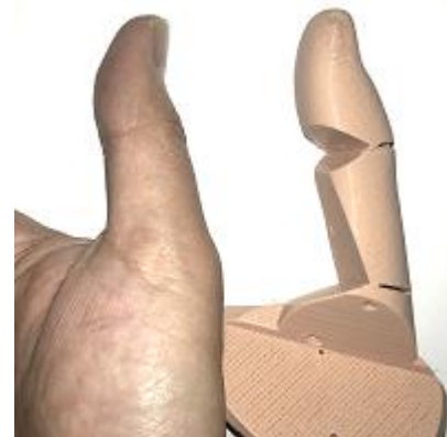
Fig. 5. The 3D-printed prosthetic thumb and a real human thumb.
