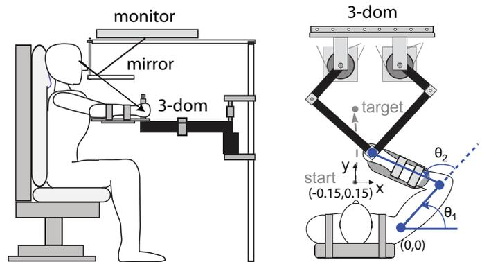
Fig. 1. Setup of the experiment: Subjects perform target reaching movements while their hand is attached to the robot, which supports the arm against gravity and can measure the hand position.
