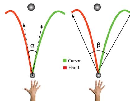
Fig. 3. Definition of angles  $\alpha$  and  $\beta$  determining the initial and final movement directions, respectively defined in equations (4) and (5).
