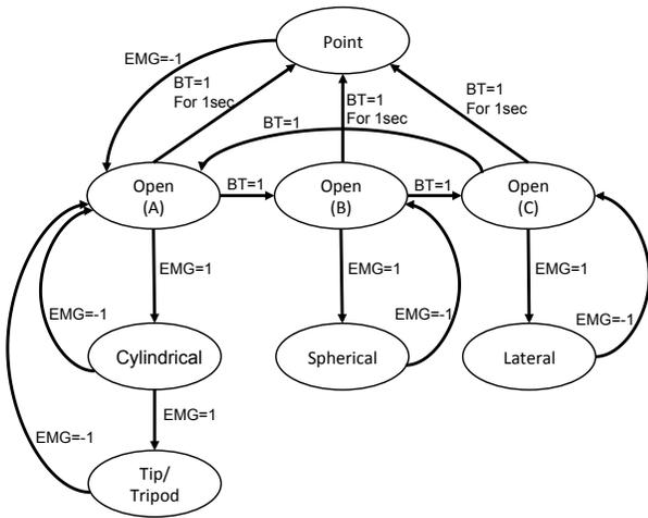
Fig. 2. Schematic of the strategy to operate the resulting hand prosthesis presented as a finite state diagram. EMG = 1 and -1 refer to actuation command from the two EMG signals, respectively and BT = 1 refers to a trigger signal
