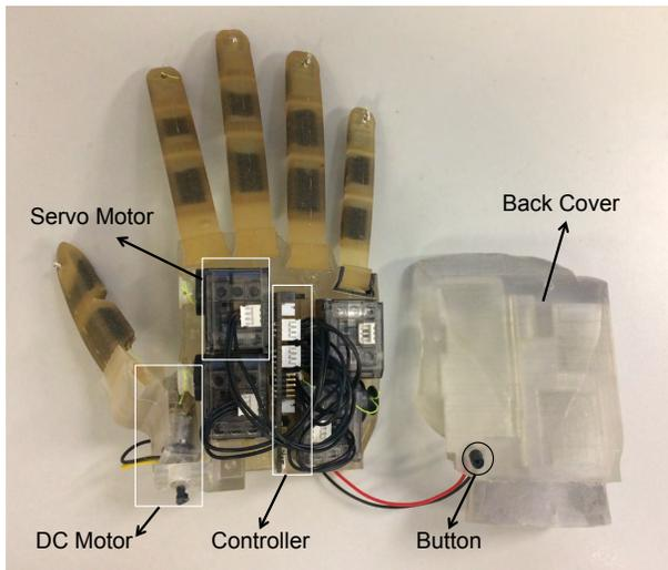
Fig. 3. Actuation configuration of the prosthetic hand prototype
