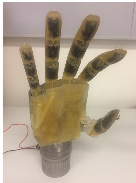
Fig. 1. Prosthetic hand prototype
