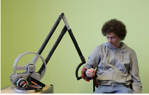
Fig. 5. The EMU backdrivable, end-effector based device for upper limb rehabilitation
