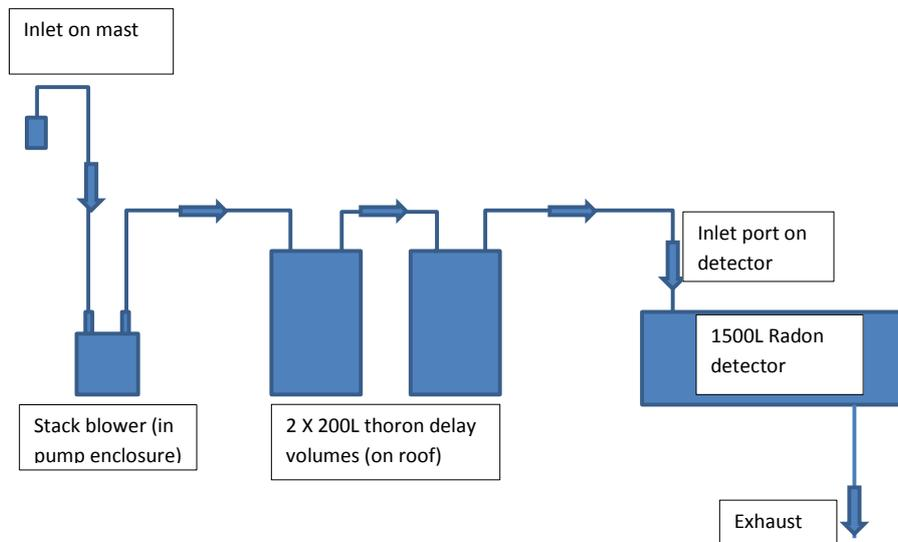
**Figure 5:** (top) Thoron delay volumes of the 1500 L AIR-BOX radon detector located on the roof of the container; (bottom) flow schematic of radon detector inlet lines and thoron delay volumes
