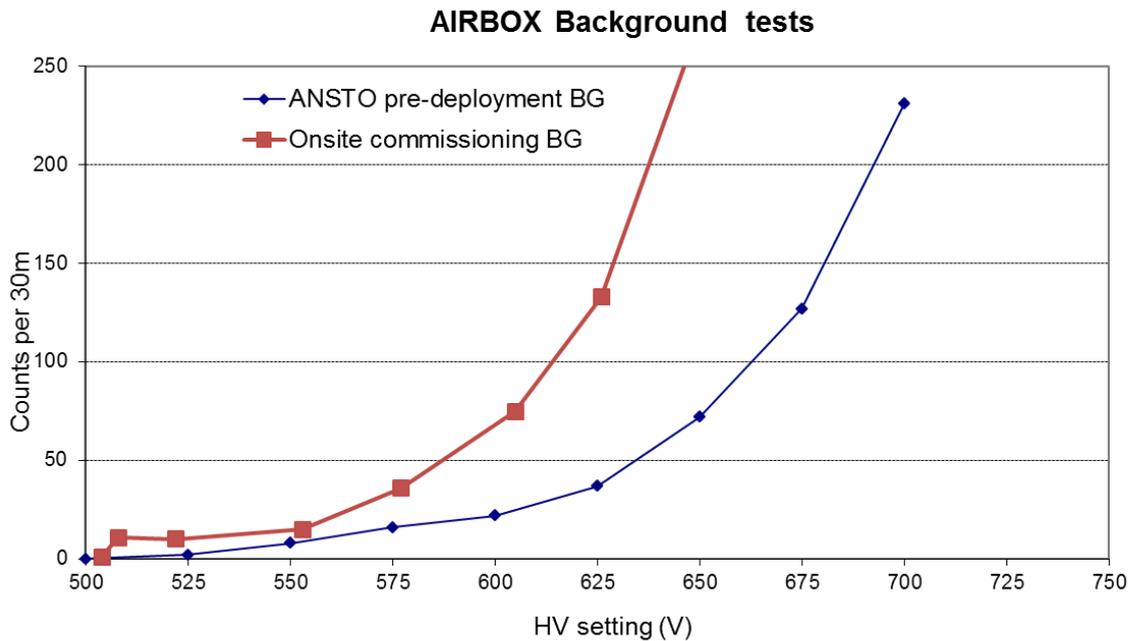
*Figure 33: Results of pre-deployment and commissioning background tests.*
