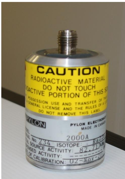
*Figure 34: Pylon “passive” calibration source for the AIR-BOX radon detector.*
