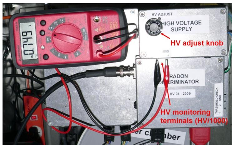
*Figure 32: Adjusting and monitoring the high voltage setting during a background check. Here the voltmeter leads are connected to terminals provided to monitor the high voltage signal (output HV/1000).*
