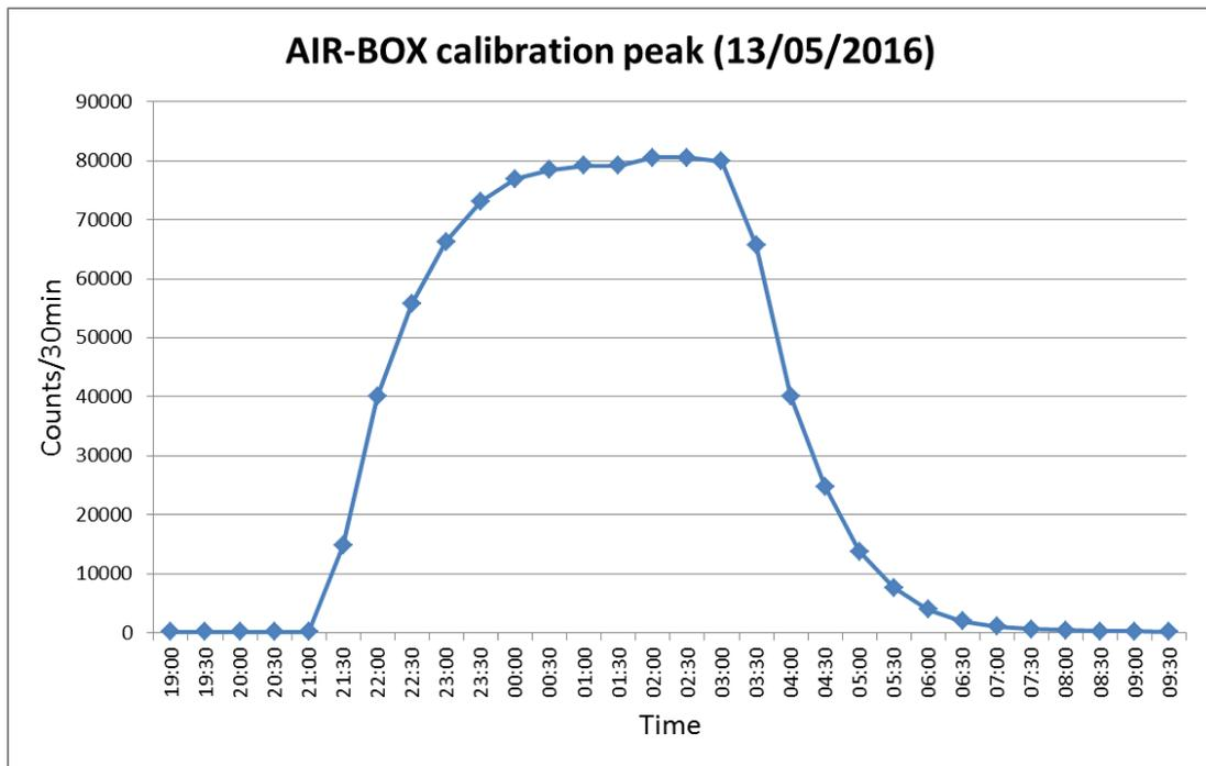
Figure 38: The first calibration curve for the AIR-BOX radon detector.
