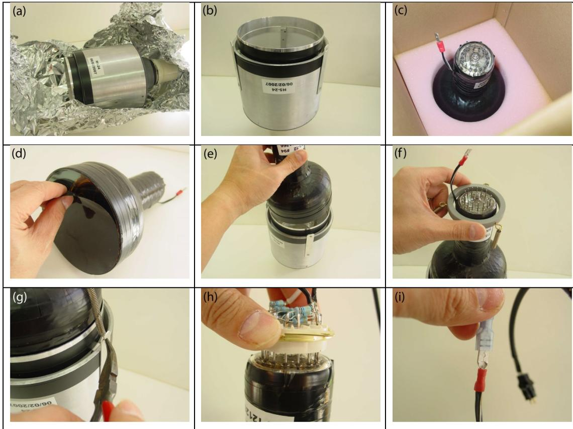
*Figure 22: Some key steps in the assembly of a radon detector head.*
