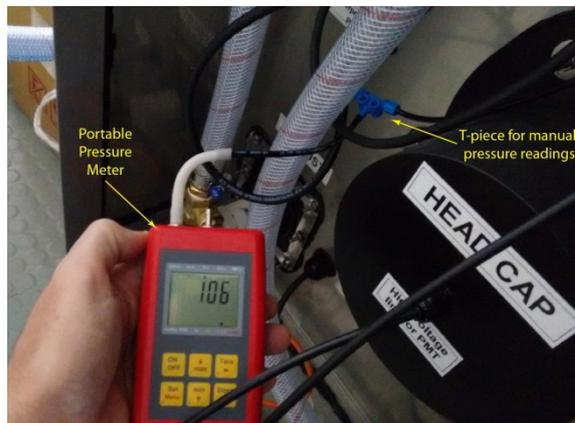
*Figure 27: Calibration of the micro mass flow sensor with a hand held differential pressure sensor.*
