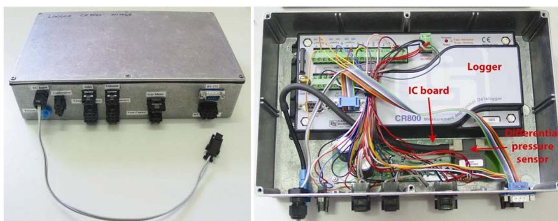
*Figure 26: CR800 data logger and auxiliary circuitry in a die-cast aluminium box.*
