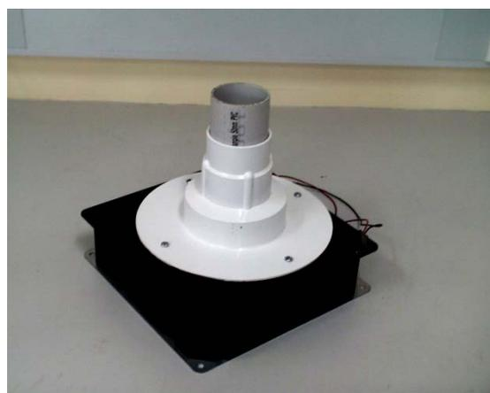
*Figure 10: Internal flow loop blower with 50mm PVC fittings.*
