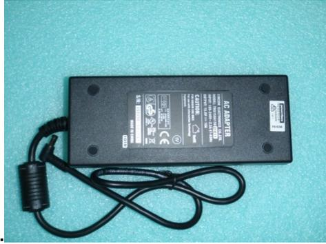
**Figure 24: Powerbox Model: TRG150A150-21E11 Power supply for the radon detector.**
