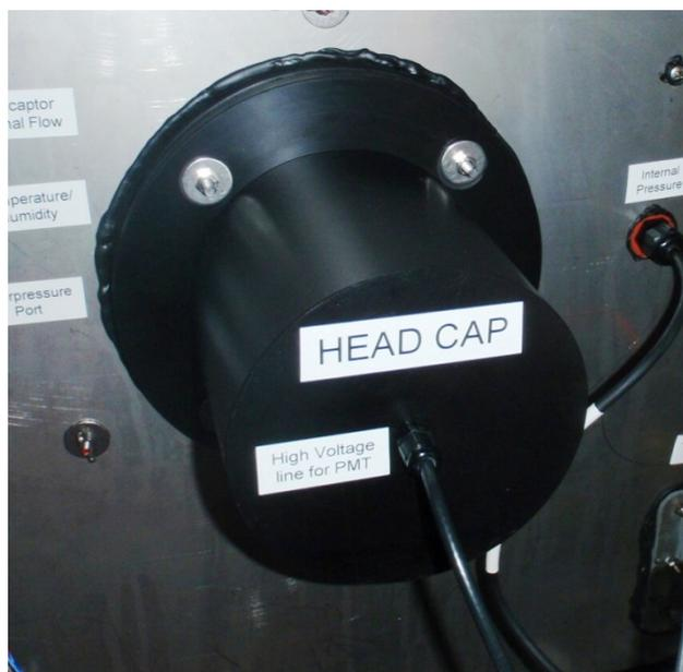
*Figure 23: Detector head cap and central high voltage cable that connects to the High Voltage / Discriminator unit.*
