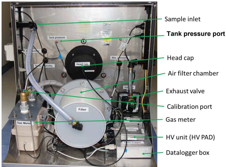
**Figure 6: View of electronics enclosure and main components.**
