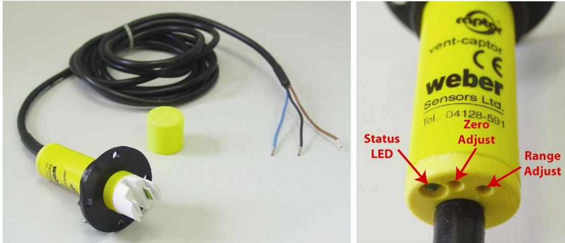
*Figure 17: Vent-captor air velocity insertion probe.*
