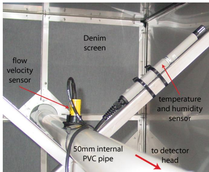
*Figure 18: Air velocity probe installed in the central pipe of the detector.*
