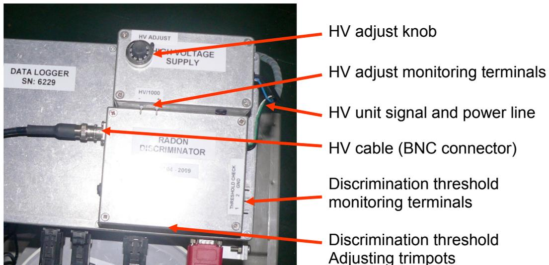
**Figure 25: High voltage / pre-amplifier, amplifier discriminator unit.**
