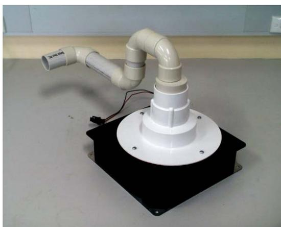
*Figure 9: External flow loop blower with 32mm PVC fittings.*
