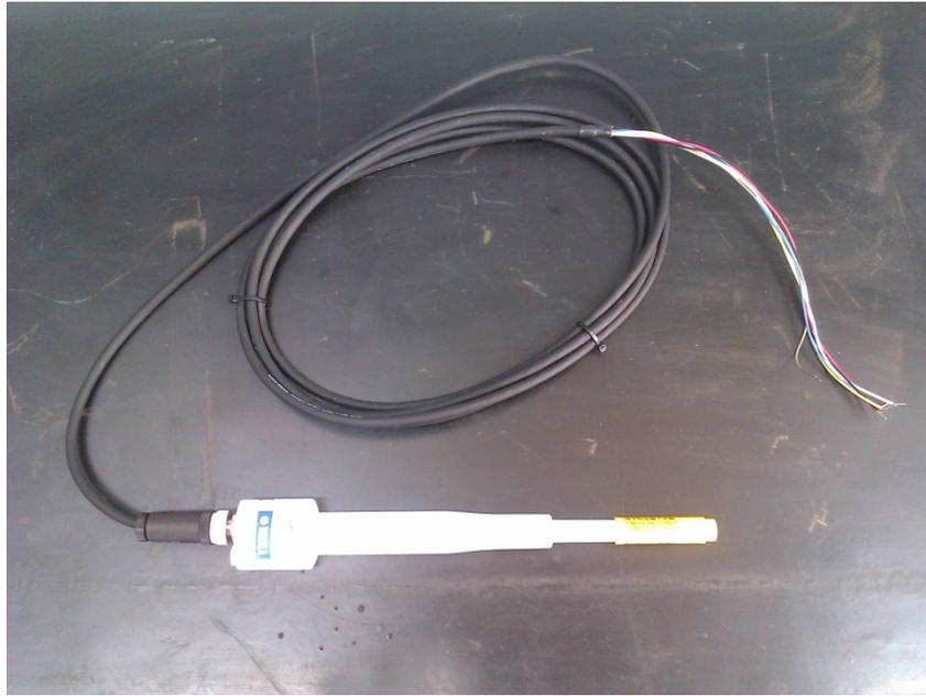
*Figure 30: Vaisala temperature and relative humidity sensor.*
