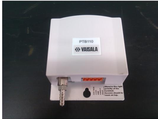
*Figure 29: Vaisala absolute pressure sensor. The sensor is mounted inside the main delay volume, so is not usually visible within the electronics enclosure.*
