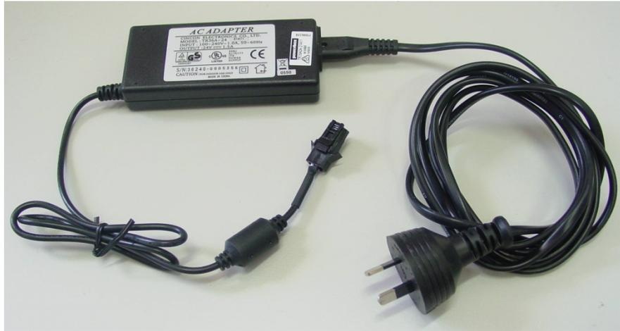
*Figure 19: Vent-captor 24 VDC power supply.*
