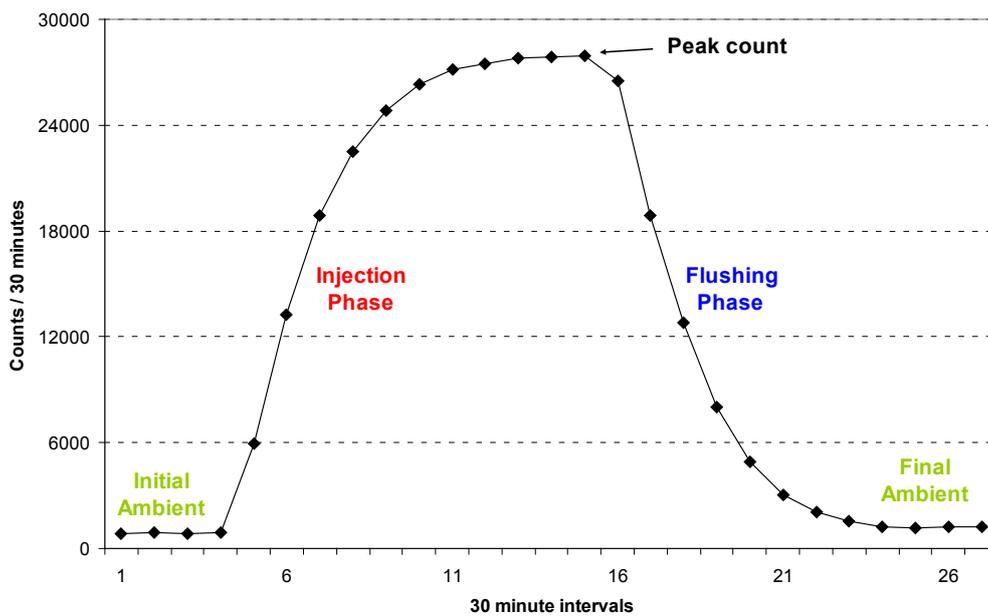
Figure 37: Example calibration event for a 1500L radon detector.
