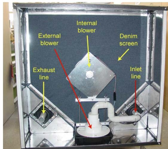
*Figure 13: View of a blower enclosure for a similar model detector.*
