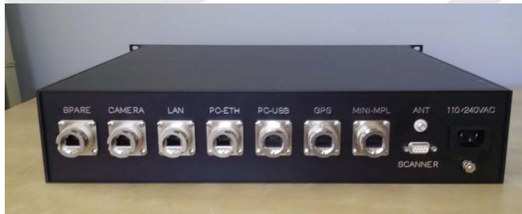
Figure 2: MiniMPL Sensor Suite Electronics Module. Rear panel showing connections.
