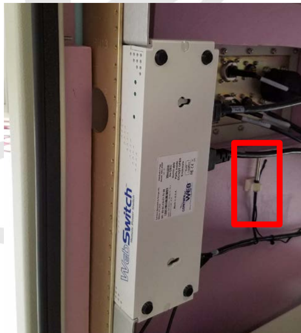
Figure 2: WebSwitch Plus™ Suggested Temperature Sensor Routing and Location
