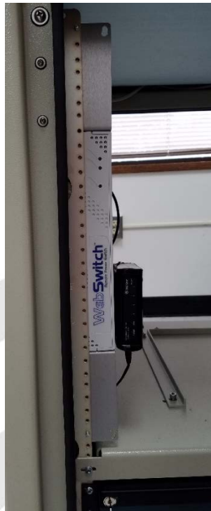
Figure 1: WebSwitch Plus™ Suggested Enclosure Mounting Location
