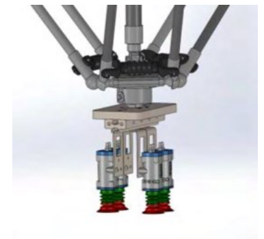
Figure 02: Prototype Robot Unit With Modified Gripper
