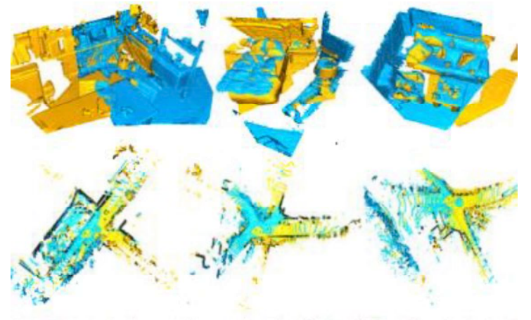
Fig. 6: The visual registration results of the proposed model on 3DMatch and KITTI are illustrated in the registratic samples. Points from the target frame are represented in blue, whereas points converted from the source frame to the target frame by the predicted transform are visualized in yellow.
