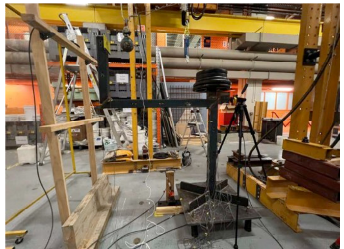
Figure 2. Setup of pendulum impact test
