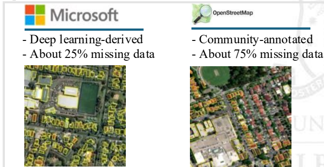
Fig. 1: Open building footprint data products in Australia and the number of missing building footprints in the study area of Chatswood, NSW.
