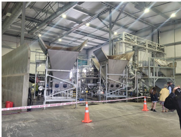
Sorting hoppers which receive and filter organic waste streams at Ecogas' Reporoa plant.
