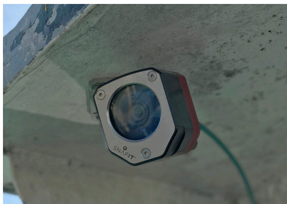
Figure 131: Camera for electronic monitoring in the fishing industry developed by SnapIT. Image credit: SnapIT.
