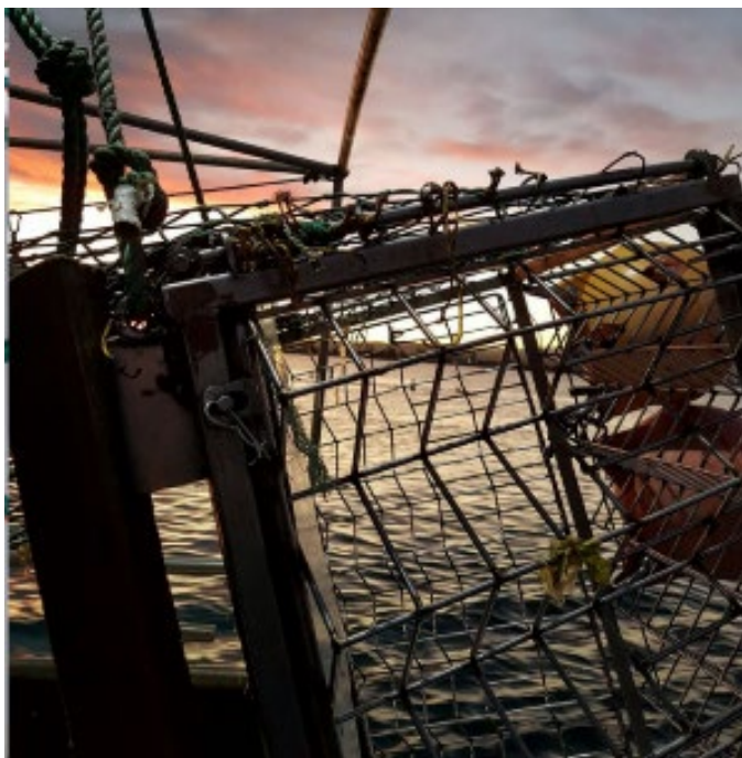
Figure 114: Rigid cod-end with rectangular openings. Image credit: Karl Warr/Better Fishing Co.
