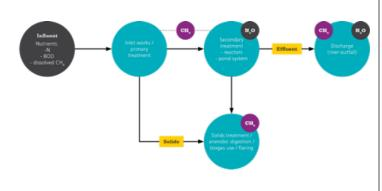
Direct Sources of Methane and Nitrous Oxide Emissions from a Wastewater Treatment Plant.
