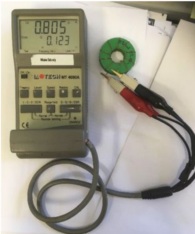
Figure 6: Measuring magnetic permeability (Low field measurement with LCR meter).
