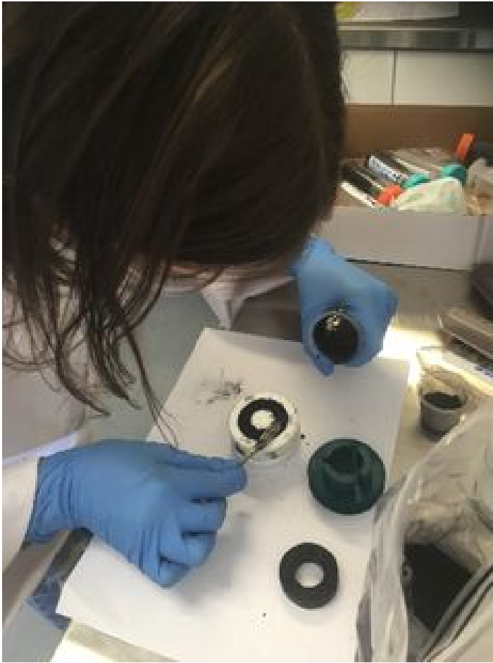
Figure 5: Making new SMC mixes of magnetic material and binder materials.
