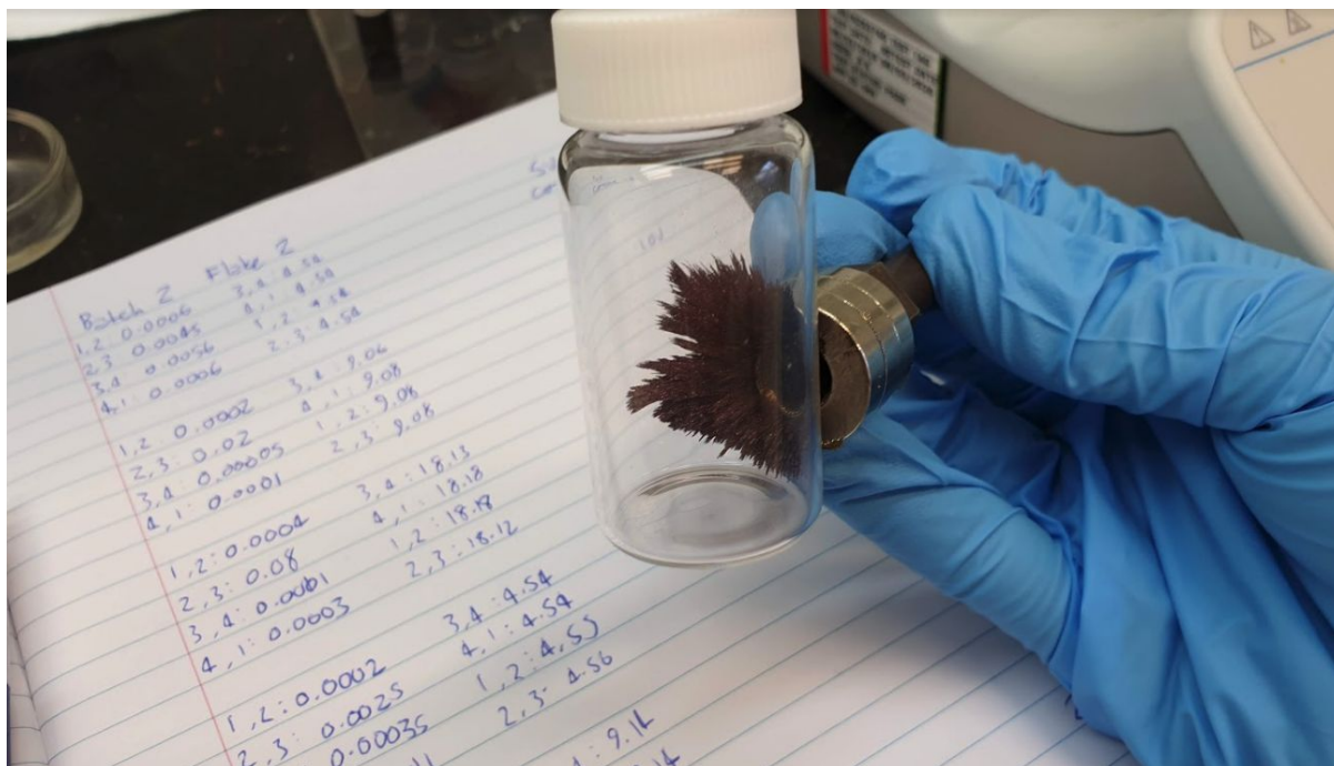
A sample of oxidised and coated Vitroperm. For use in a soft magnetic composite (SMC) which will go for magnetic testing.
