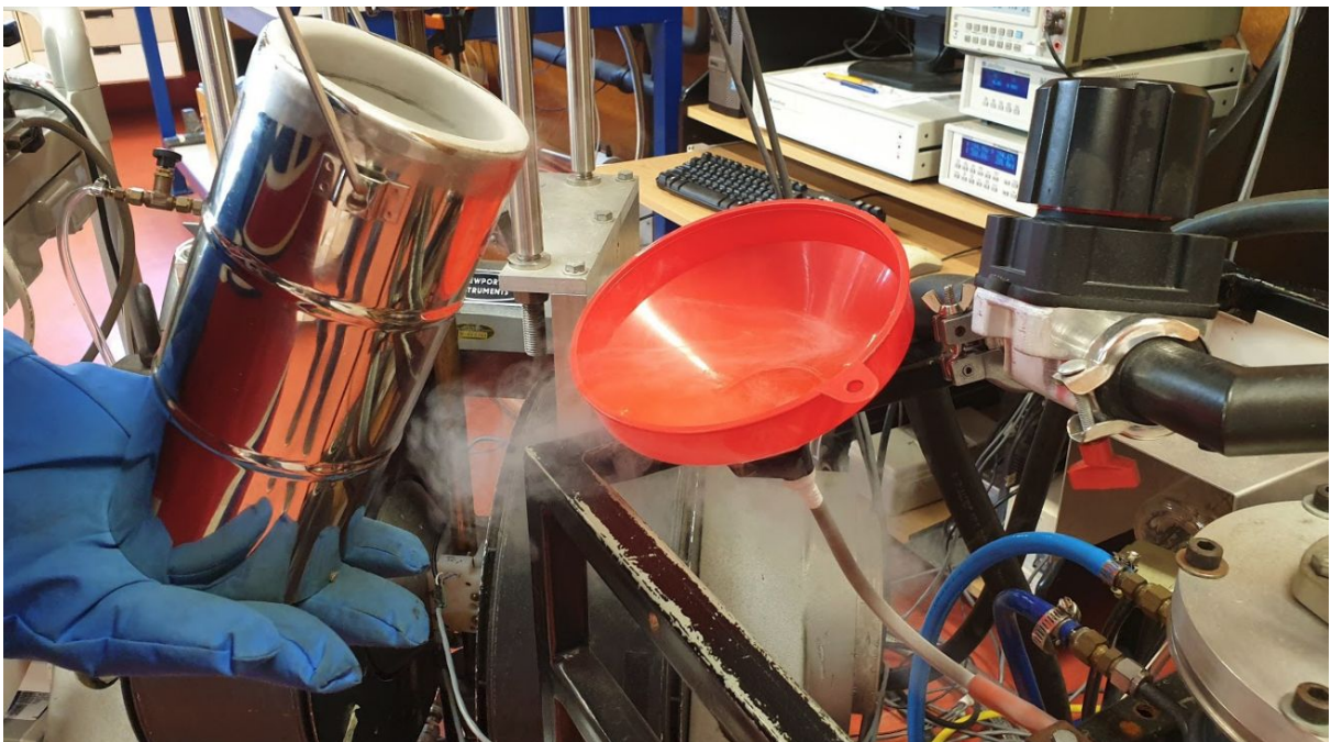
LN2 being used to cool a diffusion vacuum pump for VSM Measurements.
