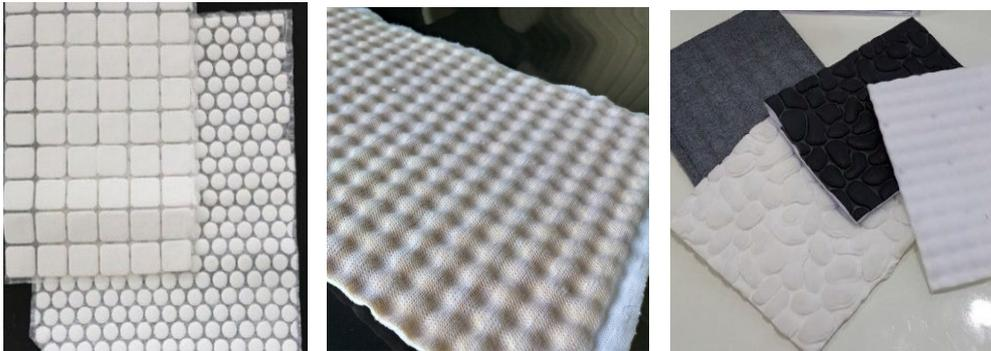
**Figure:** Various types of multi-layer laminated aerogel blankets
