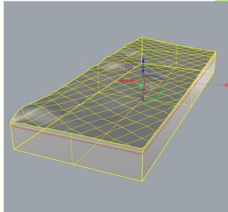
Then again using the 'Split' command, split the box using the contour surface. Remove the top of the box and you will be left with a box below in the shape of the contour. Then highlight both the surface and the box and type command 'Join'
