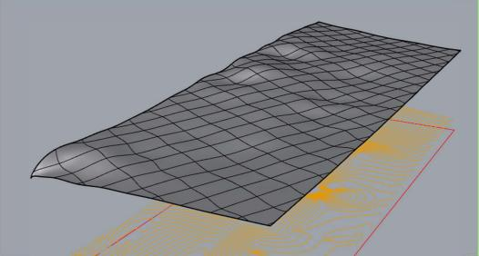
After the contour has been split, you can remove the excess surfaces outside of the bounding box.
