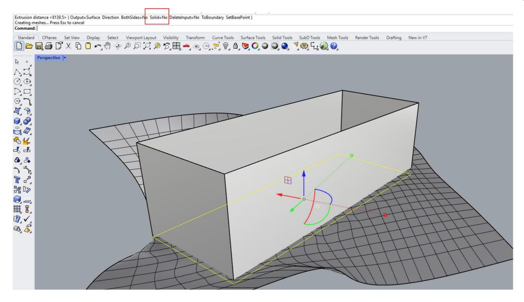
Then extrude the shape upwards, ensure that Solid=No
