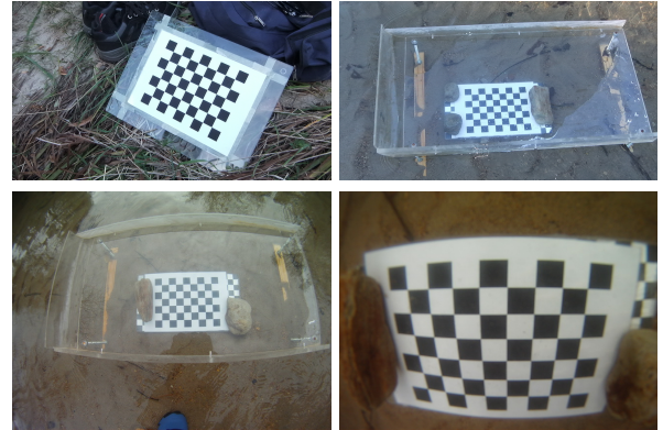
Figure 4: Example calibration image from Fujifilm W3 in air (above left), through-water (above right), GoPro Hero through-water (below left) and under-water (below right).
