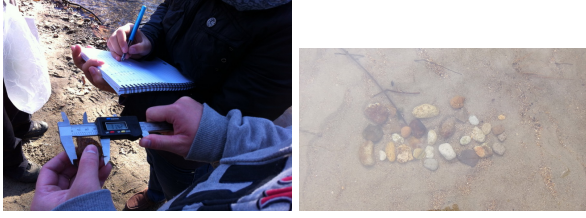
Figure 6: Pebble size measurement using digital caliper (left) and through water image of pebbles (right).
