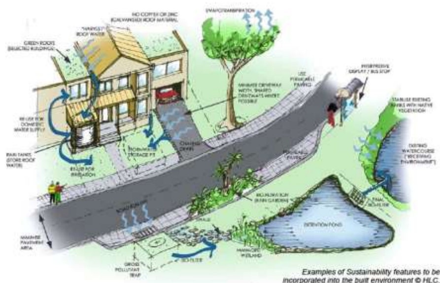
Figure 8. An illustration of sustainable water management principles to be incorporated into the comprehensive planning and design of Hobsonville Point (then name the Hobsonville Peninsula) 42 .
