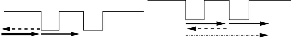
Figure 4.2. Side-view of paths for energy in grooved aluminum. Scattering of the incident surface wave causes loss of the transmitted field (left), but energy can be gained by being re-reflected in the direction of propagation (right).
