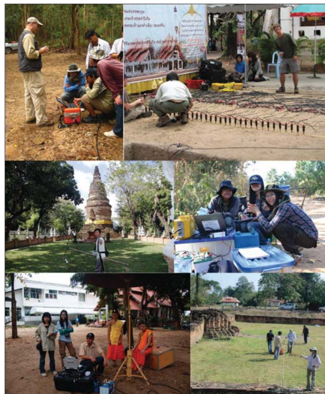
Figure 2. (clockwise from top left): Geonics ProTEM 57 time-domain electromagnetic acquisition system with instructor Rob Harris at Mae Hia; high-resolution seismic survey to map a buried wall at Wat Pan Sao; Thai and Indonesian students acquire seismic data; resistivity acquisition at Wiang Kum Kam; ground-penetrating radar acquisition with temple monk observers at Wat Pan Sao; Hoai Trung Dang collects magnetic data at Wat Pan Sao.
