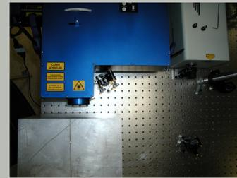
By focusing the beam of a pulsed Nd:YAG laser onto a small area of a sample, thermoelastic expansion in the sample results in broad-band ultrasonic wave propagation. A newly developed laser ultrasonic interferometer measures the absolute ultrasonic displacement for both the vertical and the radial component by collecting light scattered from the sample at high angles [2].
