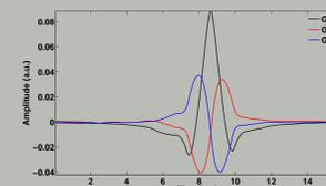
The cross-correlation between the vertical and radial components of the receivers provides an estimate of the Rayleigh-wave Green tensor. Notice the 90-degree phase shift between components.
