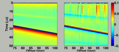
On the left, we show measurements of the vertical (left panel) and radial component (right panel) of the Rayleigh wave in an aluminum block every 0.5 mm.
