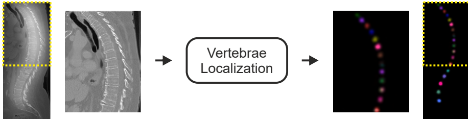
Fig. 2: Input volume and individual heatmap predictions of the vertebrae localization network. The yellow rectangle indicates that not the whole input volume is processed at once, but overlapping cropped sub-volumes. For each possible landmark, an separate heatmap volume is predicted, which is visualized with different colors.
